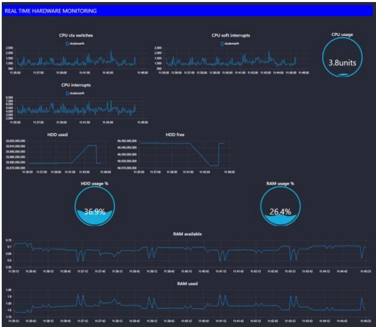
FIGURE 12 HARDWARE MONITORING AFTER A DOWNLOAD
