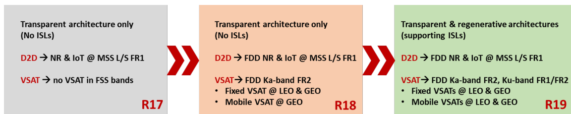
Figure 2: Satellite architectures, device types and bands in 3GPP NTN release evolution
