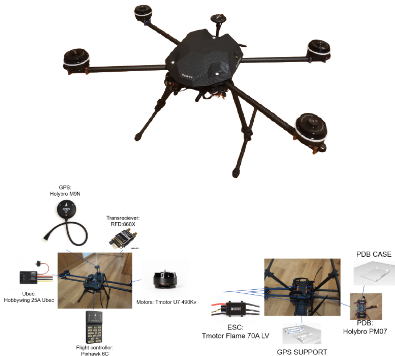
FIGURE 3. DRONE FINALLY ASSEMBLED (TOP); COMPONENTS AND TOP VIEW (BOTTOM LEFT), AND COMPONENTS AND BOTTOM VIEW (BOTTOM RIGHT)
