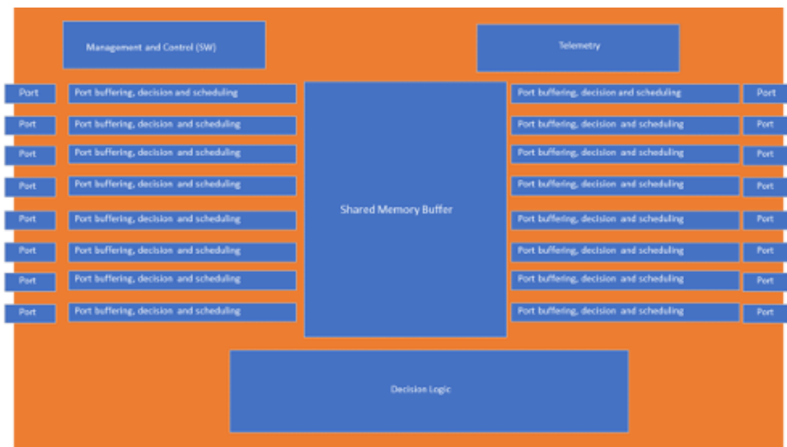
Fig. 4. Block diagram of a shared-memory switch.
